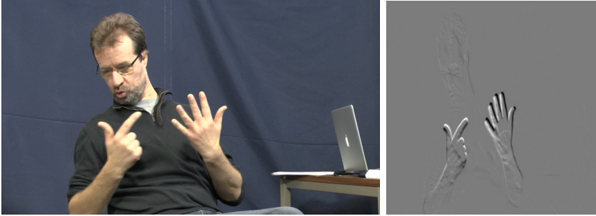
Figure 5.6: Left: Original RGB-data. Right: Model input. The RGB channels are converted to gray-scale, resized to 128x128 pixels and the previous frame is subtracted from the current frame to remove static information.
